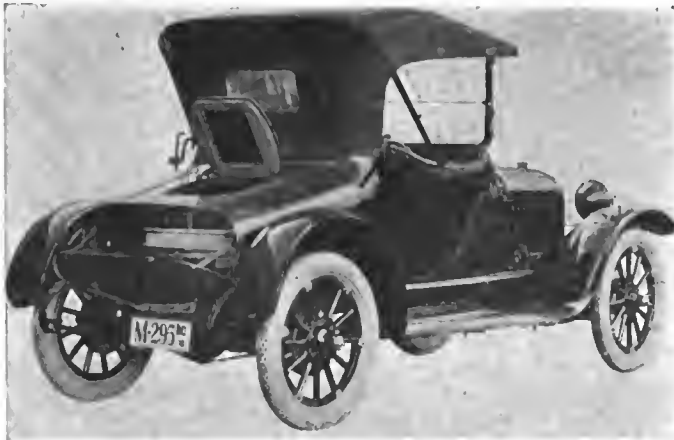
Above — Inter-State roadster, showing easy access to compartment under rear deck for tires, tools, etc. Mechanically the car is practically unchanged for 1917
